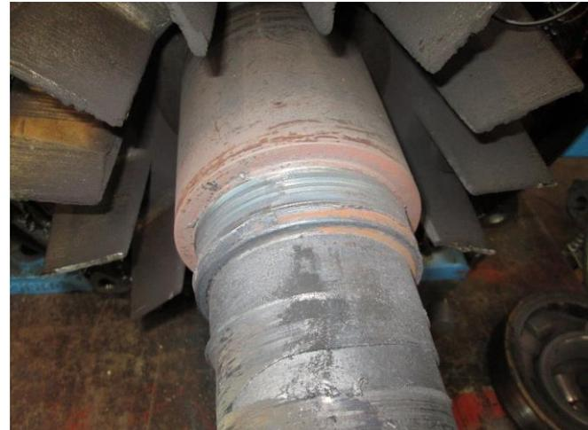
**300 HP Motor w/ roller bearings. Ball bearings were specified.**
