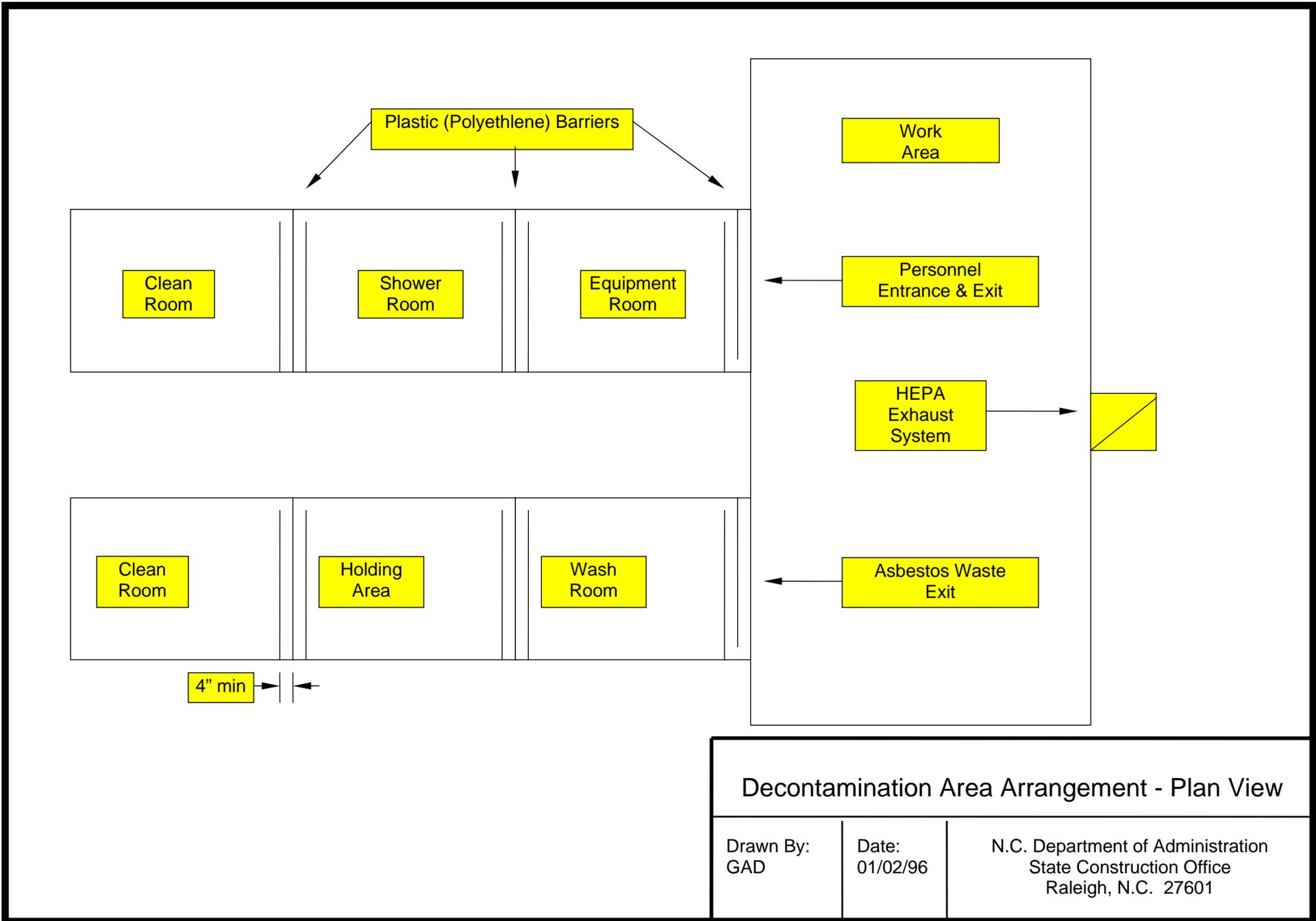
Decontamination Area Arrangement - Plan View
