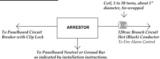
NOTE: Securely mount transient arrestor in accessible junction box or other proper metal enclosure adjacent to the panelboard, and provide engraved label indicating its location
